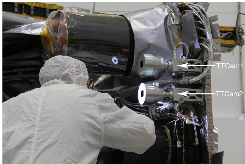
Figure 1. The two TTCam camera heads on the Lockheed Martin-built Lucy spacecraft at the Astrotech testing facility in Florida, being inspected by Ryan Bronson of Collins Aerospace, the manufacturer of the TTCam optics. For scale, each camera's semi-conical sunshade is \approx 15 cm long. Lockheed Martin photo PIRA #SSS2023010009, used with permission. Photo credit: Michael Ravine/Malin Space Science Systems.
