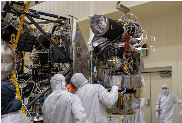
Fig. 7 Photo of the Lucy TTCam1 (T1) and TTCam2 (T2) flight cameras (with red “Remove Before Flight” covers) installed on the spacecraft’s Instrument Pointing Platform. The large cylinder to the upper left of T1 is the L’ORRI telescope (L), and the smaller black cylinder below T2 is the telescope for the L’TES infrared spectrometer (TES) [see Olkin et al. (2021) and Good et al. (2022) for additional instrument and spacecraft details]. Photo taken in Aug. 2021 at Lockheed’s pre-launch integration facility at Cape Canaveral, Florida, and used with permission of Lockheed
